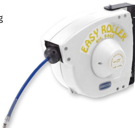
Automatic rewind, spring-driven hose reel, with plastic enclosure (made of nylon and polypropylene) suitable for the use with compressed air and water at low pressure (temperature range: -10°C – +60°C)
